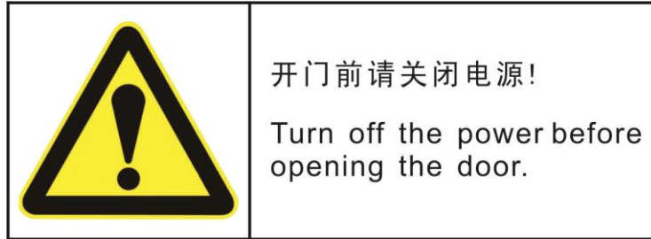
Figure 2-7 Door-opening power-off & maintenance signboard
