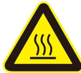
Figure 2-8 High temperature sign on control cabinet
